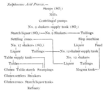
I have indicated the points at which the sulphurous acid is added, and will say in this connection, that considerable latitude is allowed. The numbers prefixed to the shakers refer to the number of the bolting cloth used.
